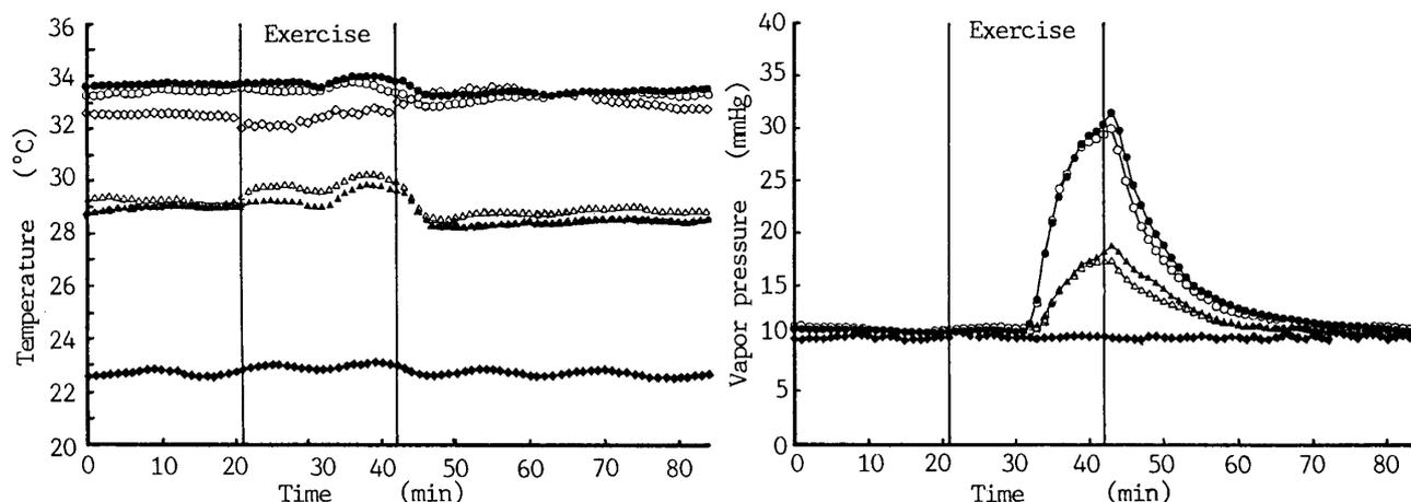
Fig. 1 Temperature and vapor pressure in the microclimate of the highly wettable shirt worn by subject S. (Sample 1)
